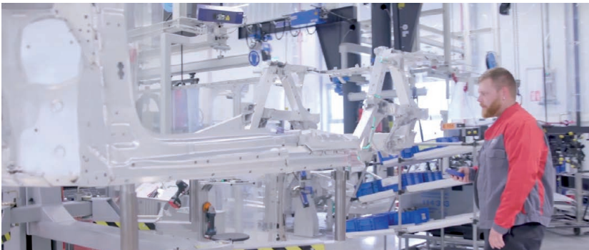
During the quality control, the employee in charge clicks on the remote control of the laser system through individual steps of the inspection, similar to a PowerPoint presentation. (Source: Z-Laser Optoelektronik)
