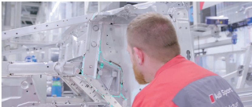
Using a defined, standardized test procedure each weld is always queried at the same time. (Source: Z-Laser Optoelektronik)
