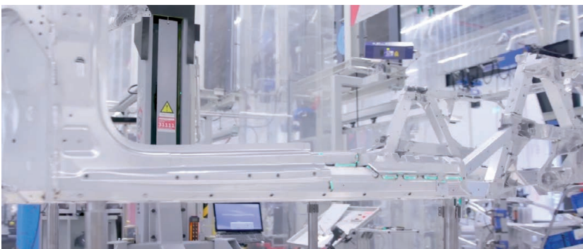
Display of welds on the body with one of the six laser projection systems in the background. (Source: Z-Laser Optoelektronik)
